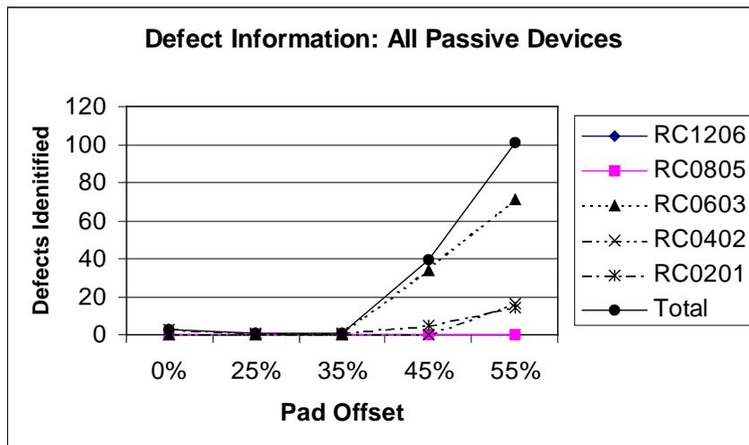
Figure 5. Number of opens as a function of offset.
