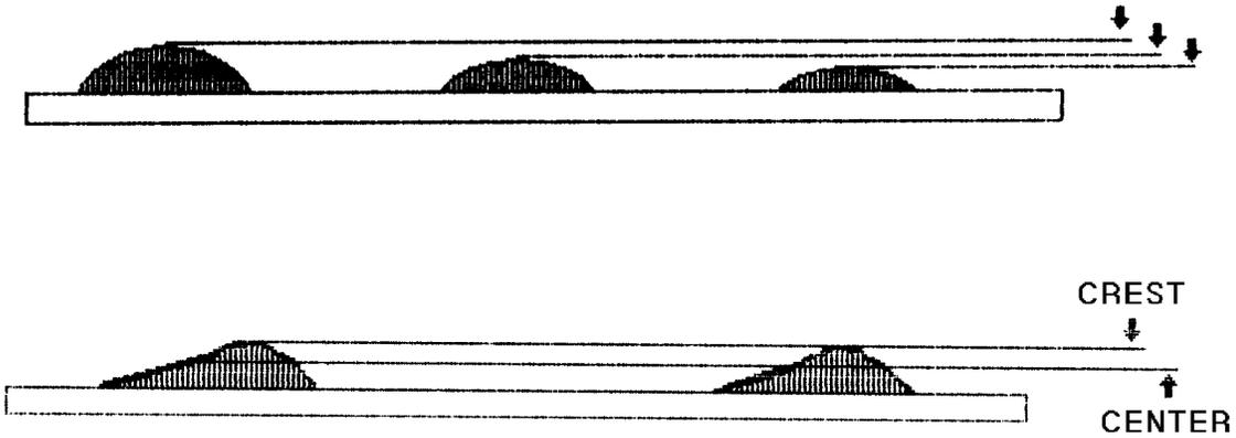
3.3 CREST: Highest point for a given feature (PAD). Since the process is geometrically dependent, smaller features on a given panel will tend to have a crest at the center of the feature. Larger features will tend to have the crest off-center as shown in Paragraph 3.1 (CENTER). This is due to normal surface tension and wet-back characteristics of the copper and solder.
