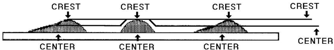
3.2 COPLANARITY: Levelness from PAD to PAD over entire board, or within certain feature size groups. This data is particularly helpful in determining thickness variations by feature, used in determining solder paste dispensing volumes for component placement.
