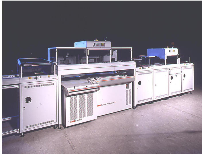
Fig. 5 – When Integrating ATE systems, you have the choice of adding a handler to an existing system (middle) or purchasing a completely integrated system (right). There are several factors to consider before you make your decision. (Photo courtesy of ITE)
